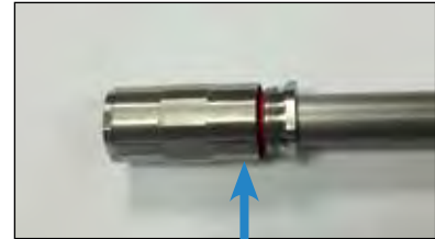
Disassembly : 2. Put the red dismounting ring on the pipe and re-screw the nut on the fitting.
