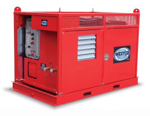
Unit is fitted with a tandem or dual stage pump. When the Pump Control Valve is in the closed or "casing tong" position (small ¼"control valve located on the side of the tank), the pump automatically transitions from approx. 50 GPM at 1100 psi to approx. 25 GPM at 2000 psi.
