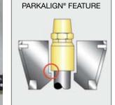
7. Rest bottom of fitting on die step using PARKALIGN° feature.
