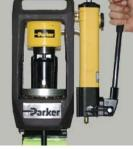
8. While holding hose and fitting into position on die step, begin pumping hand pump until die ring contacts base plate.
