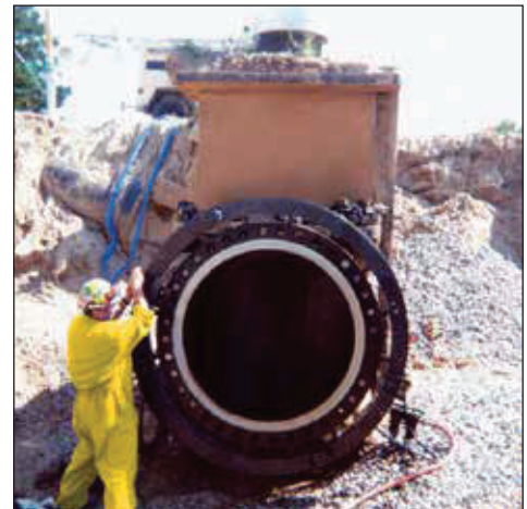
▼ HD-model heavy-duty clamshell cutter.
