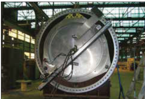
▼ Wind tower machining with WP4600.
