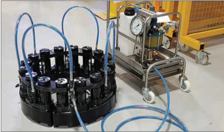
▲ Multi Stud Tensioning Set-Up.
