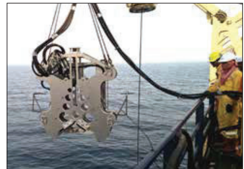
▲ MDWS Diamond Wire Saw lowered into sea.
