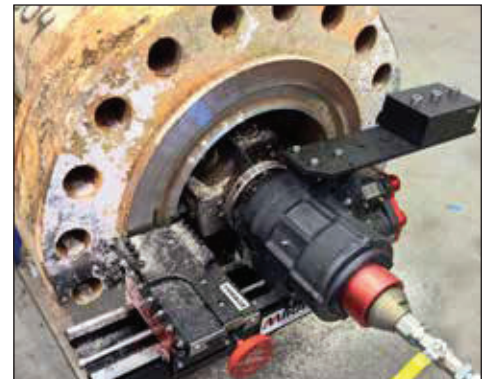
▼ MM860I machine to ensure flange joint integrity.
