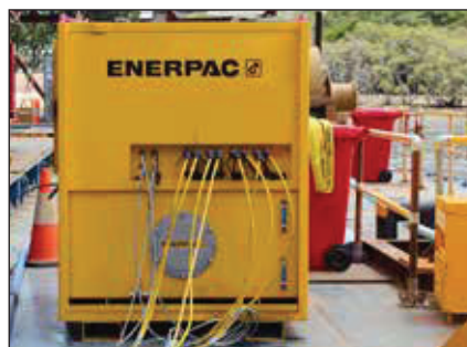
▼ SyncHoist Powerpack to operate the 4 lifting points.
