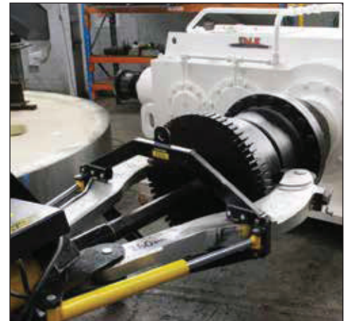
▲ The EPH1002 quickly and easily removes this drive coupler from its shaft.
