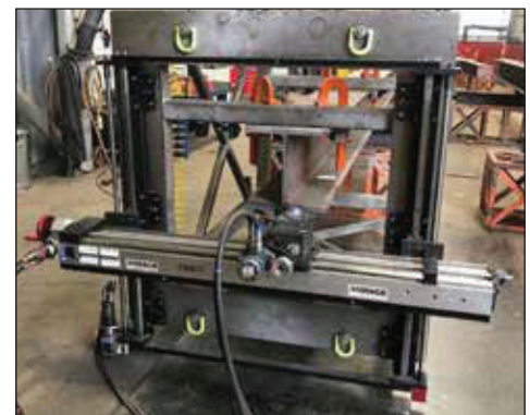
I-Beam end face milling with a GMRF1000. ▶
