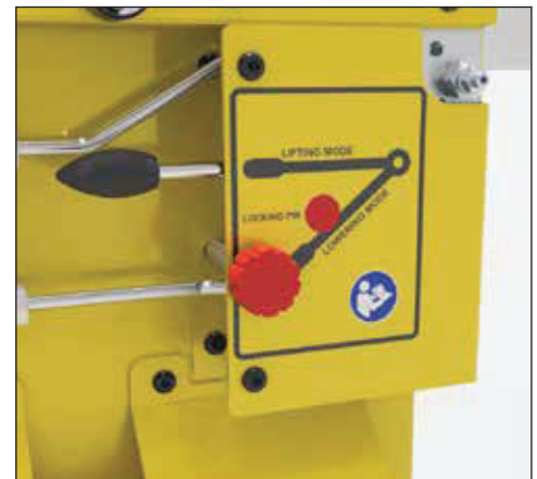
▲ Cube Jack close-up of lifting and lowering valving mode and lock handle.
