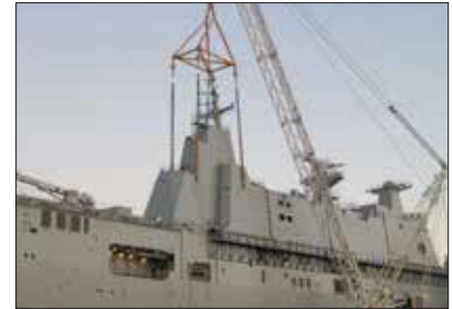
Synchronous hoisting and load positioning
