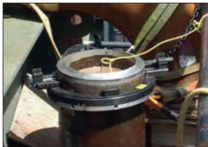
◀ NB-model narrow body clamshell cutter.
